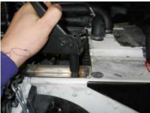
7. Install the intercooler the same way you did to check it. Do not worry if it does not feel secure the gas tank will hold it in place in a way that it cannot come off the throttle bodies.
