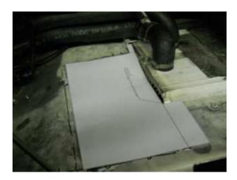
2. The template rests against the tunnel cooler. Mark with a sharpie around the outside of the template so that you know where to cut. Then using whatever tools are available to you cut out the hole. Be sure to cut it as close to the size of the template as possible. If you cut it too large you may not be able to rivet the bracket to the tunnel. If you cut it to small the intercooler won't fit down inside. Also make sure to remove the rivet on the end of the heat exchanger.
