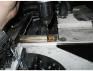
6. Rivet the bracket on starting with the front. Then pull the bracket down and rivet on the back. Make sure it is in the same location as it was when you marked it. The bracket will flex into position.
