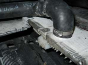
3. Check the fitment of the Intercooler mounting bracket and make any clearance adjustments necessary. Also, you may have to file down some of the high spots on the factory welds on the tunnels heat exchanger.
